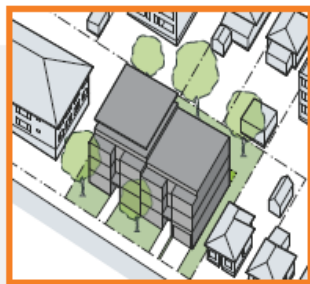
Row apartment types are modular and can be adapted to fit various site widths. They are well suited to wide, shallow lots and typically have 2-3 apartments accessed off one common access core
