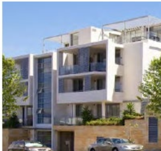
Row apartment types are modular and can be adapted to fit various site widths. They are well suited to wide, shallow lots and typically have 2-3 apartments accessed off one common access core
